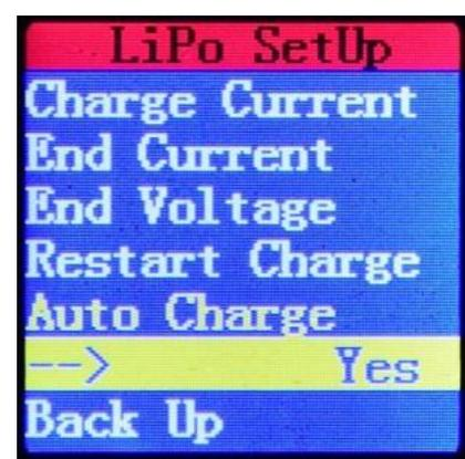
5. Press **knob** shortly can choose Battery type; press again on Battery type such as LiPo can enter into LiPo charge setup interface. Here, you can setup cell count, charge current, charge terminal current, and charge terminal voltage per cell, and then press **knob** for 3 seconds start charging.
