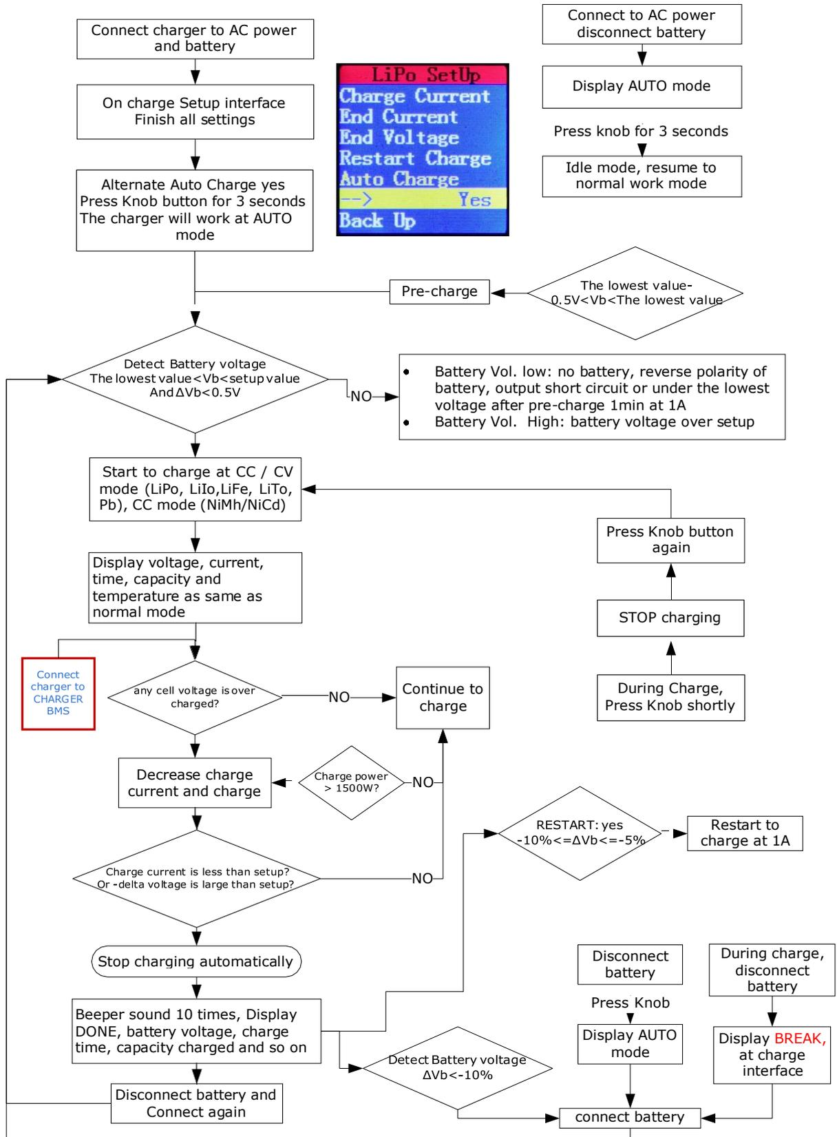
1. Connect SV102 to AC 110 / 220V outlet by the special heavy power cable, if use other brand cable, please note the wire AWG must be AWG14 at least.
